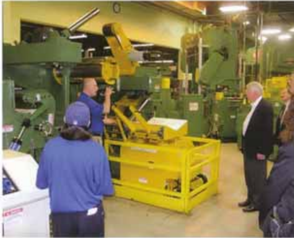
Manor employees demonstrate to Manor guests the newly installed Coe Servo-Feed line on Manors 400 Ton Draw Link Stamping Press. This feed line enhances Manors coil change capability from 20 min. to under 8 min.
